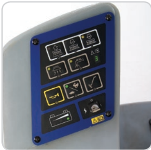
One-Touch™ activation of scrub system. All systems start and stop with machine motion.
